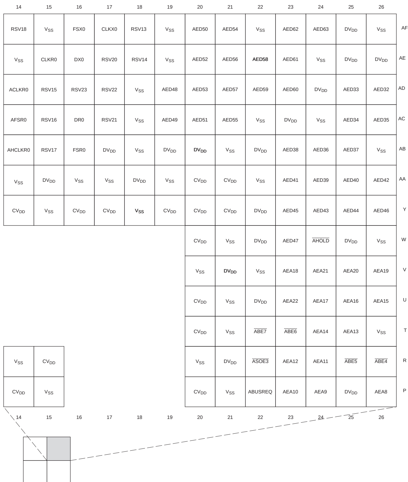
Figure 2-4. DM643 Pin Map [Quadrant B]
