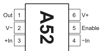
Figure 4-1. OPA300, SOT-23 Package, 6-pin (Top View)
